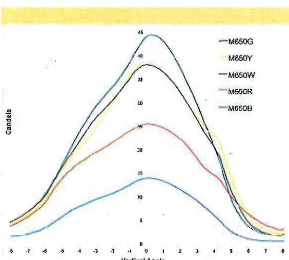
Note: Peak IALA Intensity dependent on location. Plot based on equatorial location of 12-hour night duration and 21% duty cycle flash code.
